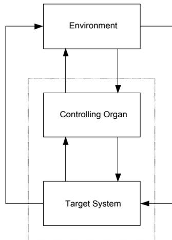
Figure 2-4: Simple control system [LEE 1994].
